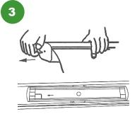
While holding the graphic firmly, remove the locking key from the end plate. Allow the graphic to slowly retract into the base. Place the key into the plastic trim of feet.
