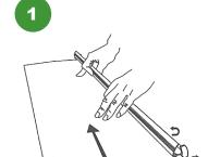
Rotate the cover of the clamp top trim, insert the top of the graphic into the clamp top trim, and then close the cover. Esure the graphic is securely attached.
