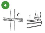
Rotate stable feet 90° and remove the pole from the banner stand base.
