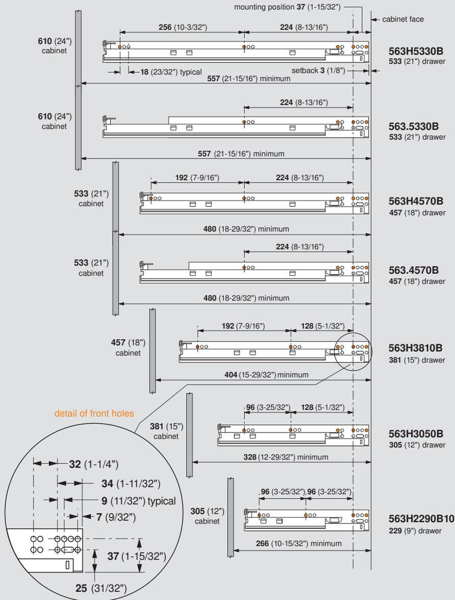
**NOTE:** Orange dots indicate screw locations required to meet specified load capacities
