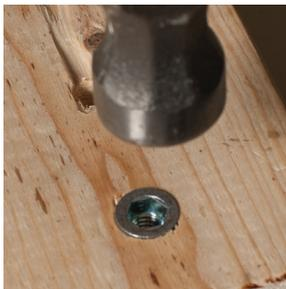
Replace with a  $\frac{5}{16}$  -18" threaded insert nut. Use a hammer to tap in the insert nut.
