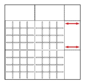
Position the ceiling tile and firmly hold it in place, making sure that the adhesive makes good contact with the ceiling surface for proper adhesion.
