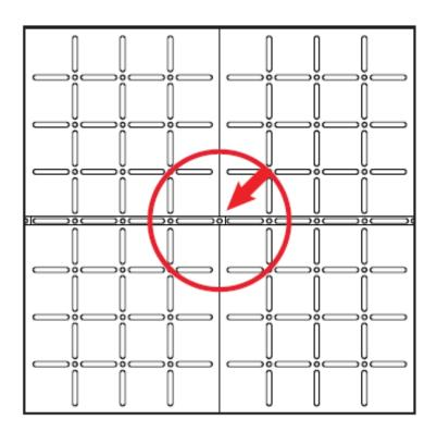
Butt the next decorative strip directly against the end of the first, creating a repeating pattern - the first dot on the second strip placed over the next four-way ceiling tile intersection. Again, dry-fit and trim as necessary.
